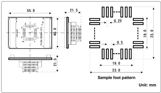
Figure 5.2 External dimensions of the FLX-144NSD
